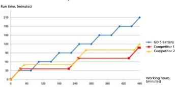
All horizontal lines indicated charge times for battery and diagonal lines show runtime GD 5 Battery run time = 43% of an 8 hour cleaning.
