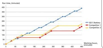
All horizontal lines indicate charge times for battery and diagonal lines show runtime GD 5 Battery run time = 81% of an 8 hour cleaning
